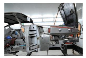
Objective – to remove all components, filth, materials, coverings and paint which are required prior to separation of the outer body shell from the chassis assembly. First stage of the strip is to remove all interior trim and glass, labelling and carefully storing. Next follows bumpers, all bright trim, light fittings etc. Next the transmission tunnel was removed followed by the removal of radiators, engine and transmission in unit, initially to be stored and later assessed.
