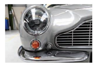
It is Aston Workshop policy that after a total restoration, any car being prepared must have undertaken at least 500 miles to shakedown, reveal any defects and undertake final testing and tuning. Such was undertaken with this car. No major problems were encountered and only minor adjustment to idling speed and final tune was required to create a smooth and tractable driving experience.
